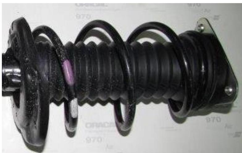
Slika 14 Vzmet prednja os / Figure 14 spring front suspension
