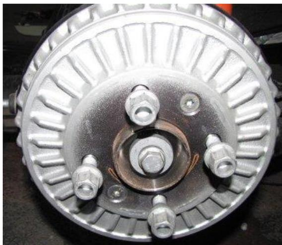
Slika 23A – zadnji zavorni koluti – 237 ali 273mm / Figure 23A - rear brakes – 237 ali 273mm
