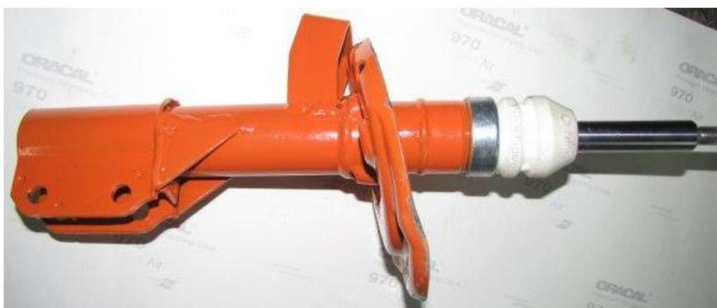
Slika 20 – prednji amortizer / Figure 20 - front shock absorber
