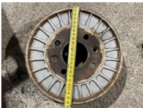
Slika 23B – zadnji zavorni koluti – 237 ali 273 mm / Figure 23B - rear brakes – 237 or 273 mm
