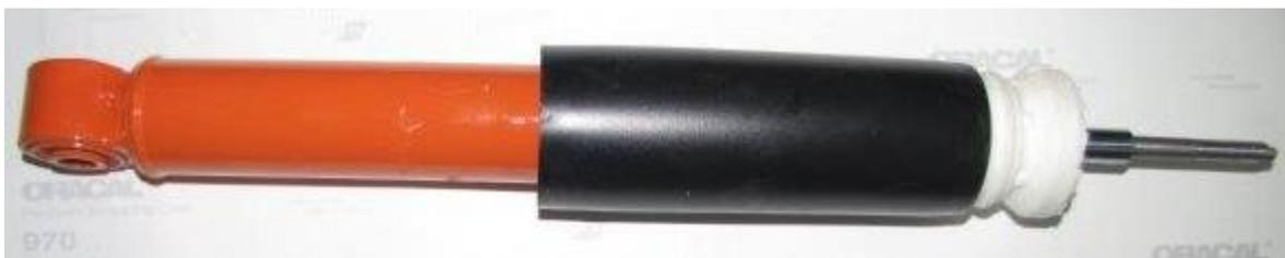
Slika 21 – zadnji amortizer / Figure 21 - rear shock absorber
